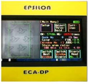
Deployed300mm from its target, an ECA-DP with 8mm lens inspect for verification of presence of release paper on sanitary pad.
